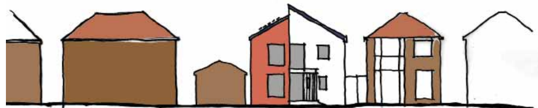
Street elevation (early sketch)- materials to be self coloured render with blue black eternit slates and dark grey window frames Early sketch of streetscape below
