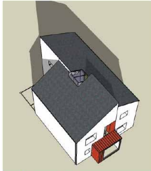
Axo - showing interlocking roofs and rooflight
